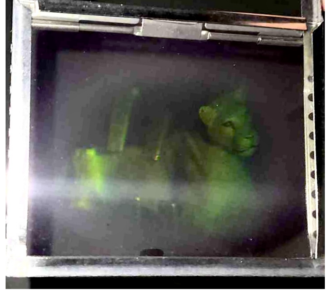
Figure 3: Experimental results showing the reconstructed wavefront of the lion object. Note the characteristic green colour, indicating the film shrank by approximately 50 to 100 nm after processing.
