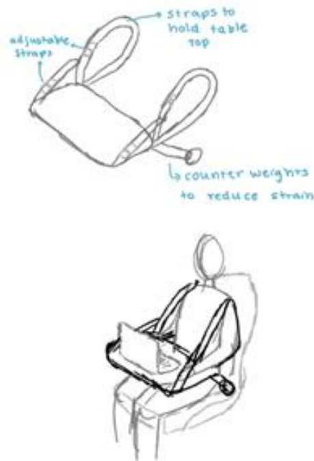
Figure 14: Sketch demonstrating the DeskPack's features and how it should be used.
